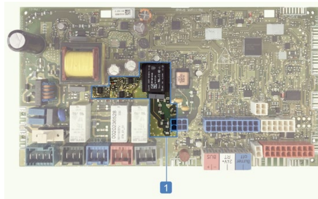
1 = Converter (ioniDETECT- Signal)
